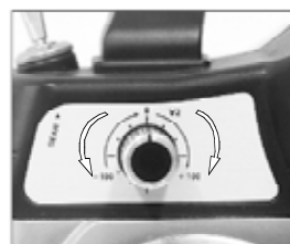
Rotating V2 leftward or rightward to discretionarily adjust the amount of PIT limitation extent.
