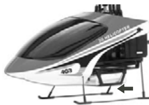
Step 3: take off the canopy and remove the battery pack.
